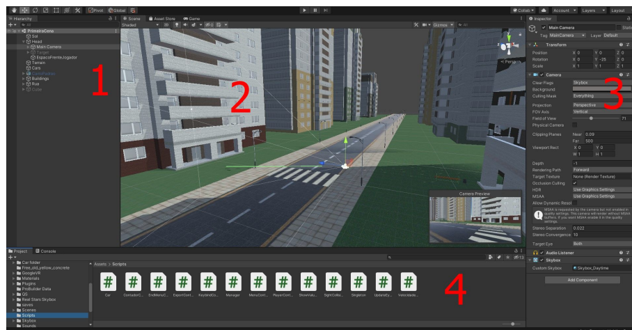
Figure 2.5: The Unity Interface. 1: Hierarchy View. 2: Scene View. 3: Inspector Window. 4: Project Window.
